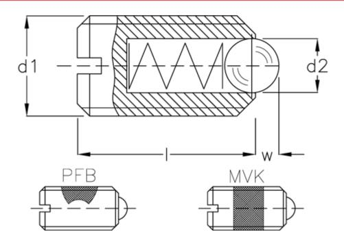
$\begin{array}{ll} \text{d1} & = \text{M24} \\ \text{d2} & = 15.0 \\ \text{Length I} & = 34 \\ \text{Spring pressure N bottom} = 237.0 \\ \text{Spring pressure N top} & = 127 \\ \text{W} & = 5.5 \end{array}$
